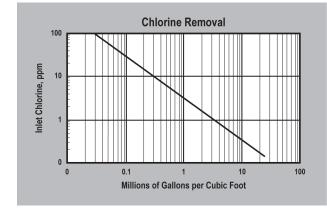
The graph above shows throughput capacity for chlorine removal using 2 gpm/cu.ft. of deionized water at  $77^{\circ}F$  with 0.1 ppm chlorine leakage endpoint.
