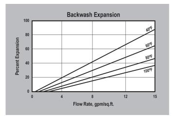
**BACKWASH** — The carbon bed should be backwashed at least once per week with chlorinated water to expand the bed 15 to 20 percent. This helps keep the carbon bed sterile and removes any foreign matter and carbon fines.
